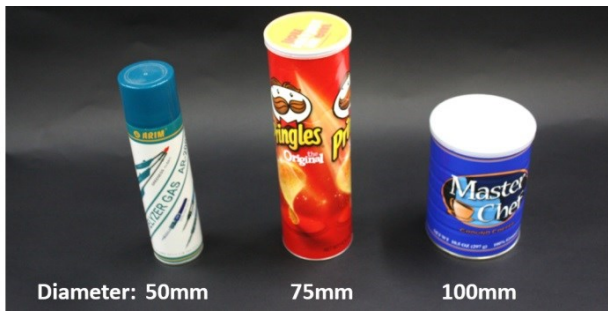
Fig. 9. Objects used for the wrap grasp force experiment.
